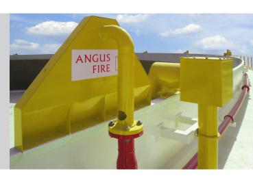
Angus Rimseal Foam Equipment is used for the protection of vertical open top floating roof (OTFR) storage tanks and comprises two elements - the Rimseal Foam Generator (RFG) which produces expanded foam when supplied with foam solution and the Rimseal Foam Pourer (RFP) which delivers the foam gently into the rimseal area.
