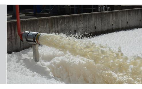
Angus Medium Expansion (MEX) Bund Pourers are designed for fire protection systems and vapour suppression on bunded or diked areas surrounding flammable liquid or toxic chemical storage tanks. They are also suited for other applications requiring large volumes of free flowing foam eg. process areas, warehousing and storage protection.
